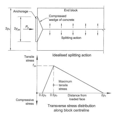
Figure **Error! No text of specified style in document.**.28: Tensile splitting stresses arising from concentrated prestressing
