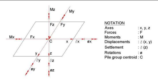
Figure Error! No text of specified style in document..25: Illustration of Pile Group Design Data
